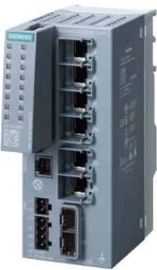
SCALANCE XC206-2SFP G manageable Layer 2 IE switch; IEC 62443-4-2 certified; 6x 10/100/1000 Mbps RJ45 ports; 2x 1000 Mbps SFP; 1x console port; diagnostics LED; redundant power supply; temperature range -40 °C to +70 °C; assembly: DIN rail/S7 mounting rail/wall; redundancy functions; office features (RSTP, VLAN,...); PROFINET IO device; Ethernet/IP-compliant; C-PLUG slot; IEEE 1588v2 PTP
