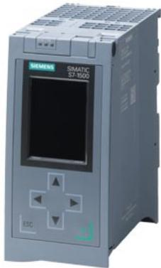
\*\*\* spare part \*\*\* SIMATIC S7-1500R, CPU 1515R-2 PN central processing unit with work memory 500 KB for program and 3 MB for data, 1st interface: PROFINET RT with 2-port switch, 2nd interface: PROFINET, SIMATIC Memory Card required
